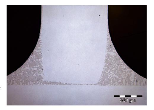
A photomicrograph of a typical brazed tee-joint. The braze filler metal was originally placed on one side of the joint and flowed through via capillary action, properly filling the small gap area and forming a smooth fillet on each side of the joint. Silicides can be seen as a result of the silicon contained in the braze filler metal used (Amdry<sup>TM</sup> 105).
