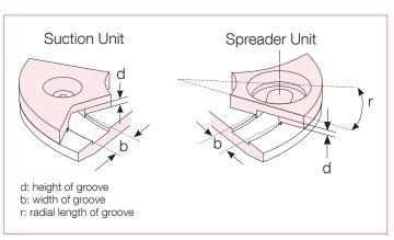
Type NL units are for non-liquid powders (powders that do not flow easily). Type L units are for freely flowing liquid powders. Additional types can be used for powders such as abradables with plastic or graphite additives or other special cases.
