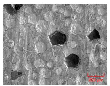
Worn surface of a Metco 81586 weld hardface.
