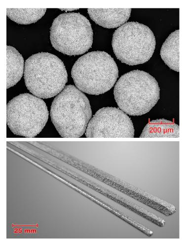
Top: SEM photomicrographs of Metco 51151B, showing morphology that is typical for these products. Bottom: Metco 81586 welding rods.
