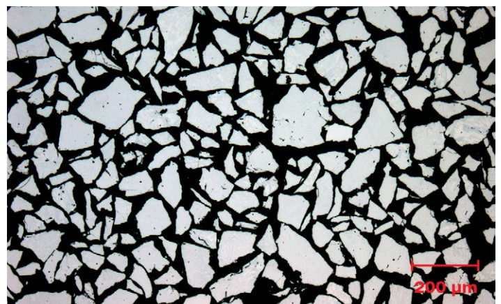
Photomicrographs of WOKA CTC. Top: Outer morphology showing irregularly shaped particles. Bottom: Inner structure.
