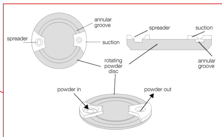
The rotating disc powder feeder uses a volumetric method of feed rate control.
