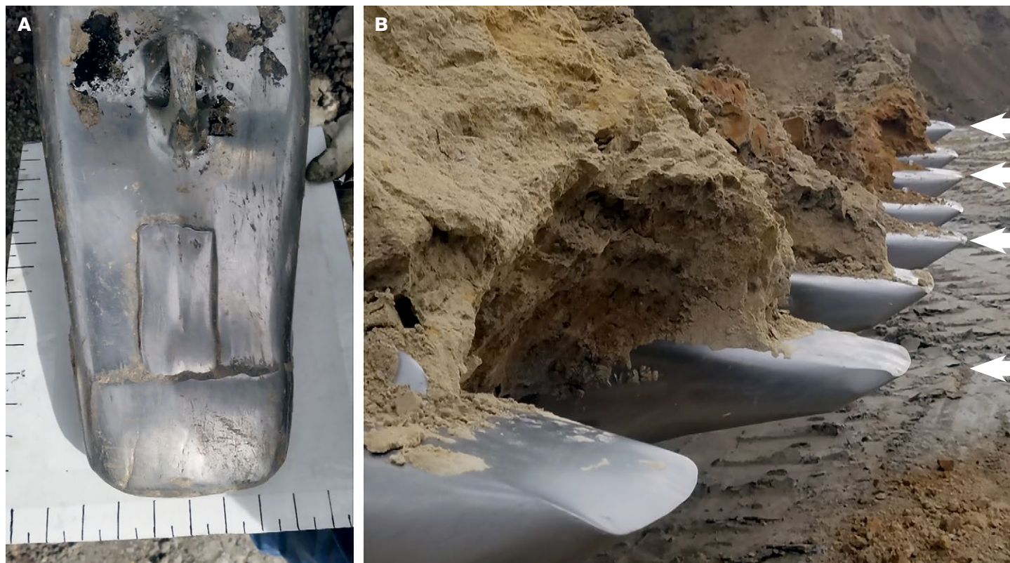
Figure 8. Trials using Metco 8247, a non-cracking hardfacing, GETs in service. A: Close-up of hardfaced GET. B: Comparison of hardfaced and unhardfaced GETs. White arrows highlight the hardfaced GETs. Notice that the hardfaced GETs are longer and less worn, attesting to the abrasion resistance of Metco 8247.
