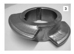
minimal pause of the process between cladding tracks. Here too, programming the cladding tracks in the CAD system is advantageous.
