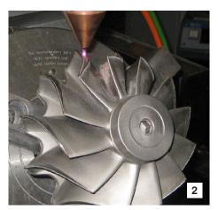
surface of the component on various programmed tracks at any angle of incidence. In the laser cladding process, the laser beam is ideally mounted perpendicular to the workpiece.
