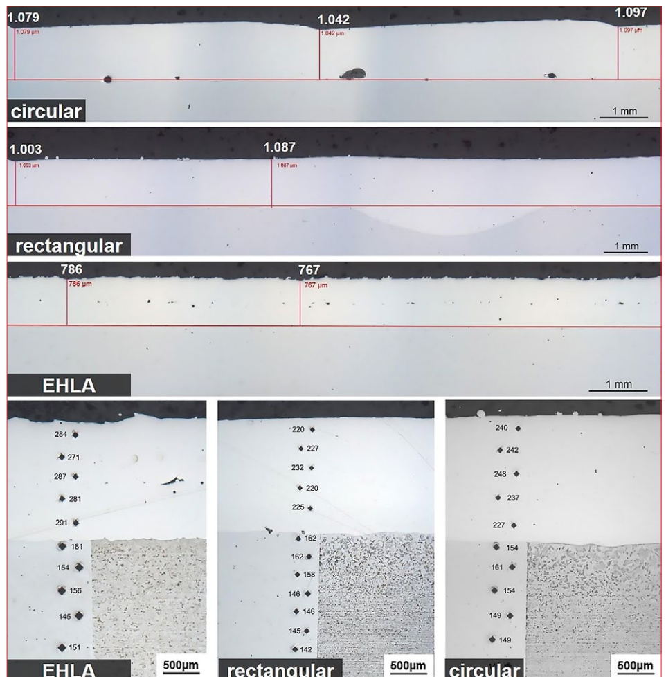
Figure 6: Cross-sectional micrographs, and hardness distribution values for tubes after laser cladding
